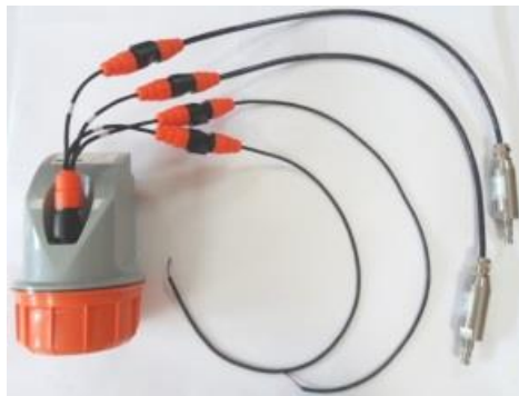
An example of an off-the-shelf cable system. This particular setup gives two analogue inputs, and two pulsed inputs
